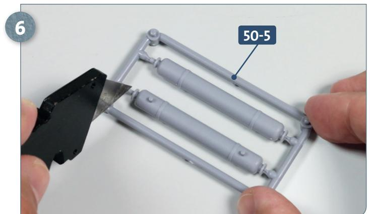
Separate both halves of the compressed air bottle from the frame **50-5**. Use some sandpaper or fine file to smooth away any remains of the attachment points.
