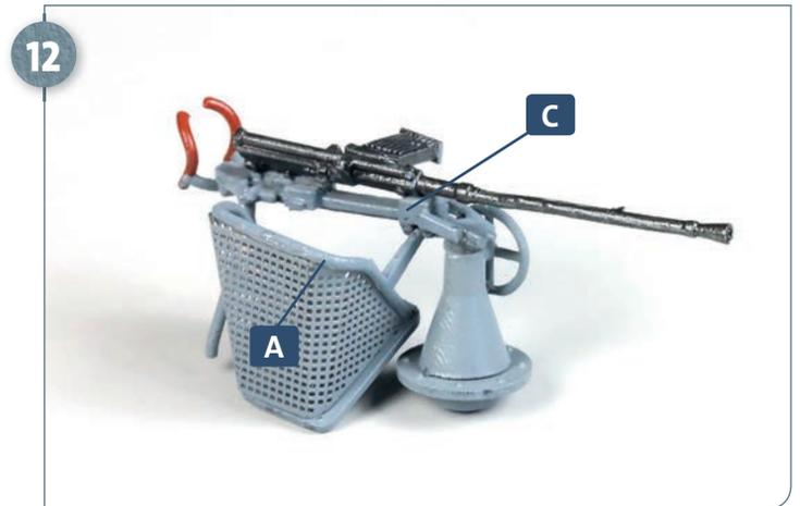
Glue the bracket A to the lower gun carriage C as shown in the photo above.
