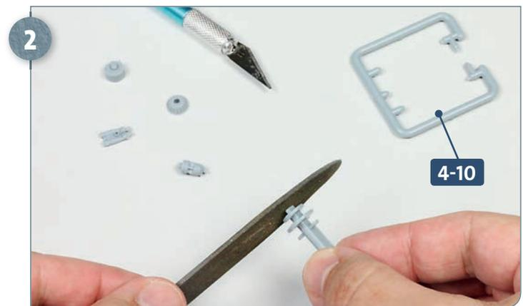
Carefully detach the five pieces from 4-10 and use a small flat file to remove the remains of the frame.
