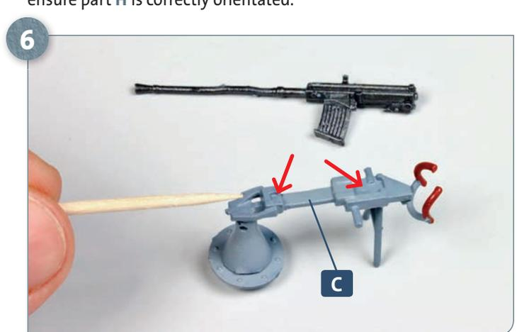
Apply a small amount of glue to the places marked by the two arrows on upper carriage **C**.
