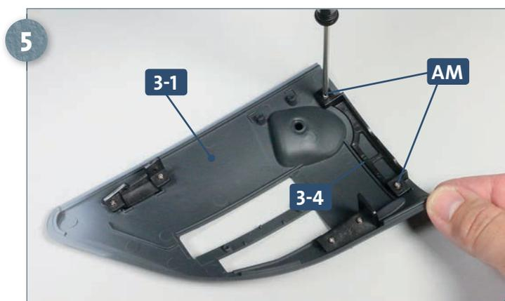
Take Hull connector **C 3-4** and attach it to the back of the bow section **3-1** using two **AM** screws.
