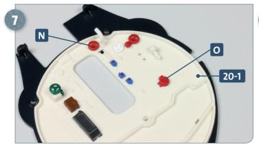
Detach the two remaining parts from frame **20-7**, **N** and **O**, and glue these to the bulkhead **20-1** as shown above.
