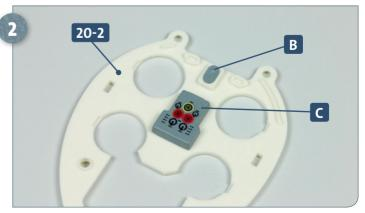
Glue part **B** into the recess at the top of the mounting plate **20-2**. Add some glue to the pegs of part **C** and glue these into the holes in the centre of the mounting plate.
