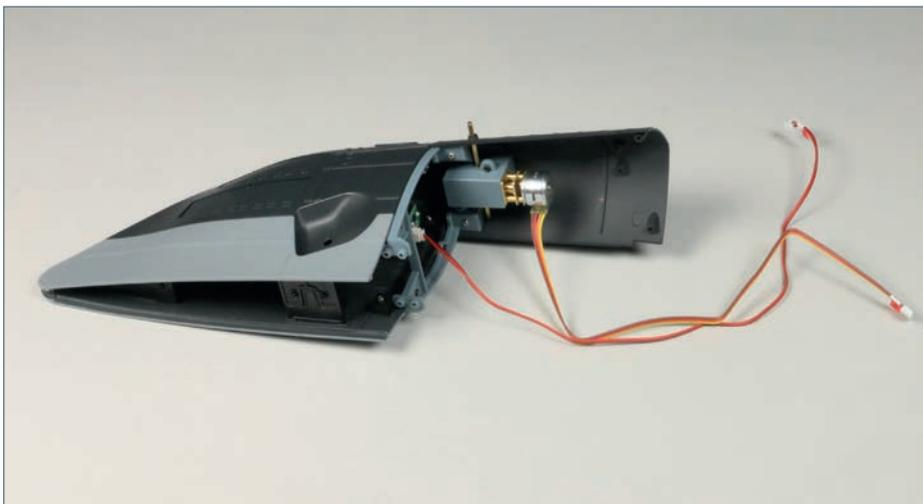
The motor for the forward hydroplane has been connected to the gearbox, and the hydroplane assembly attached to the hull.
