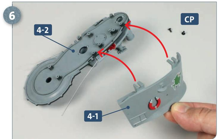
Taking care not to damage the parts, turn the port (L) bridge deck assembly **4-2** upside down. Have ready two **CP** screws. Take the bulwark **4-1** and fit its tabs over the raised screw sockets, as indicated by the two arrows.
