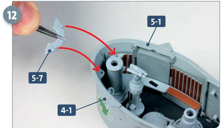
Take the canopy 5-7 and fit the two pegs on its underside into the holes inside the two halves of the bulwark 4-1 and 5-1, as shown. If necessary, use a small file, or similar, to adjust the part.
