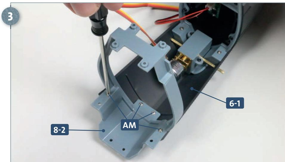
Fix the two parts together using four **AM** screws.
