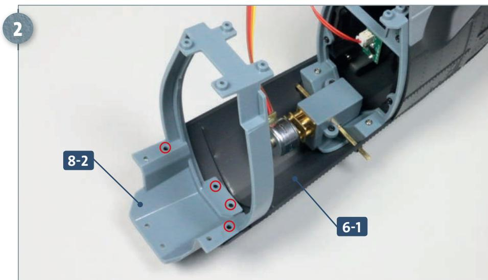
The connector **8-2** is correctly positioned when all four holes align with those of section **6-1** (circled).
