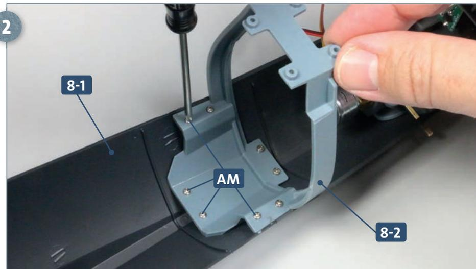
Fix in place using four **AM** screws in the holes indicated in the image.
