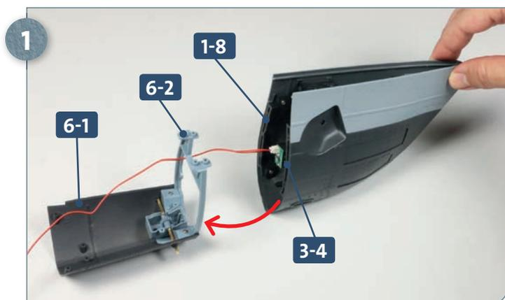
Fit the bow assembly to the new hull assembly **6-1**, aligning the holes of connectors **1-8** and **3-4** with those of connector **6-2**.
