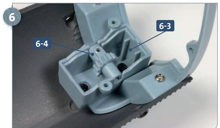
The gear **6-4** is correctly seated in the hydroplane box **6-3** when the hole on the shaft is facing upwards.
