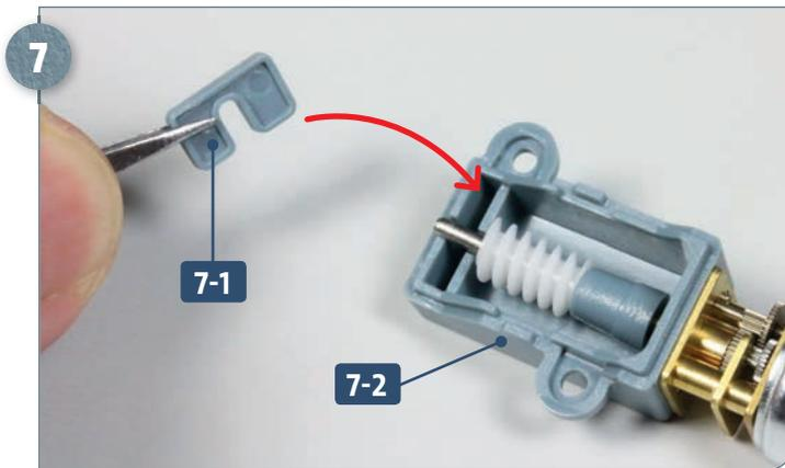
Take the bracket **7-1** and fit it onto the split recesses of the hydroplane box **7-2**, as shown. Pay close attention to the orientation of the part.
