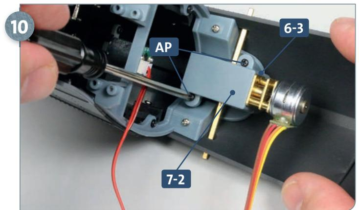
Fasten the two parts of the hydroplane box **7-2** and **6-3** together using two **AP** screws, as shown.
