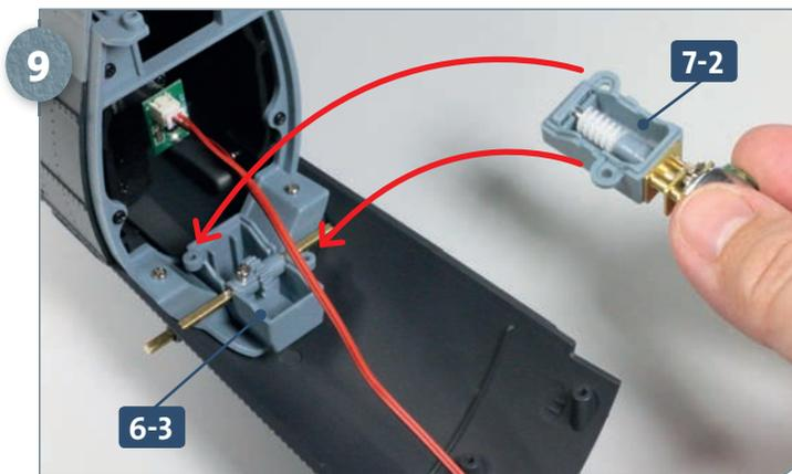
Place the hull assembly, which was worked on in the last kit, on your work surface. Fit the upper hydroplane housing assembly **7-2** onto the lower housing **6-3**, as shown.
