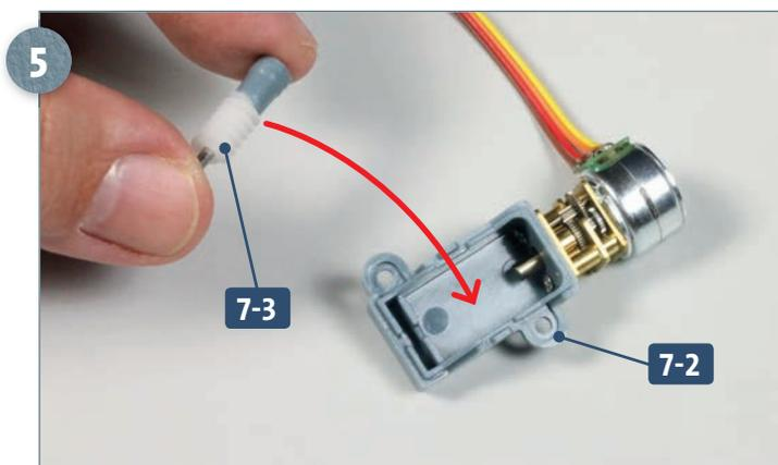
Take the worm gear **7-3** and fit it onto the shaft of the motor inside the hydroplane box **7-2**. Note that there is a flattened side to the shaft, which aligns with a flattened edge inside the worm gear.
