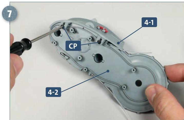
Attach the port (L) bulwark **4-1** to the bridge deck assembly **4-2** using two **CP** screws.
