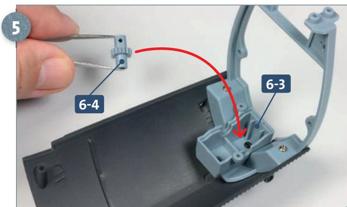
Take the gear **6-4** and insert it into the hydroplane box **6-3**, as shown above.
