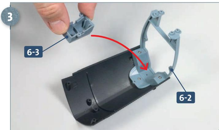
Take the hydroplane box housing **6-3** and fit it onto the connector **6-2**. Pay careful attention to the alignment, referring to the photo shown above.
