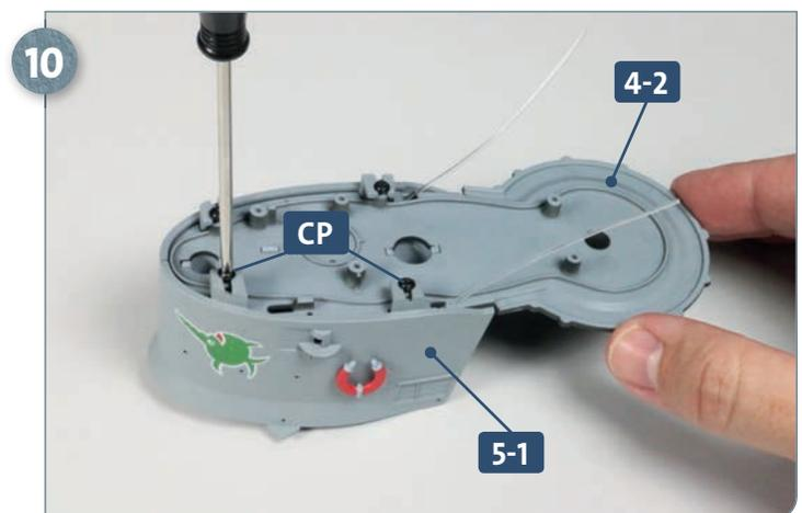
Use two **CP** screws to fix the bulwark to the bridge deck as shown above.
