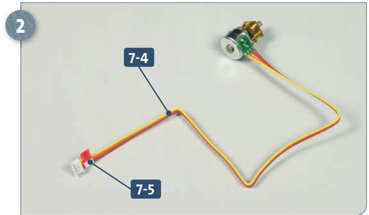
Attach the cable label **7-5** just next to the connector end of the cable **7-4**, as shown in the photo.
