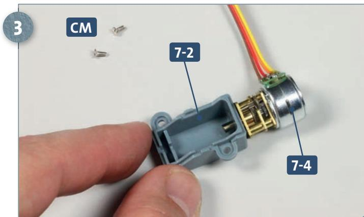
Fit the shaft of the motor **7-4** into the hole in the hydroplane box **7-2** and have two **CM** screws ready for the next step.
