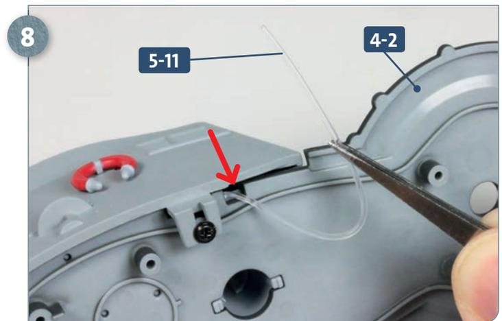
Make sure that the fibre optic cable **5-11** is routed through the gap behind the air duct cover and through the recess (see arrow) in the bridge deck **4-2**.
