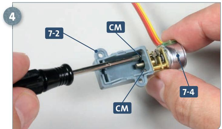
Fix the motor **7-4** onto the hydroplane box **7-2**, using two **CM** screws in the positions shown above.
