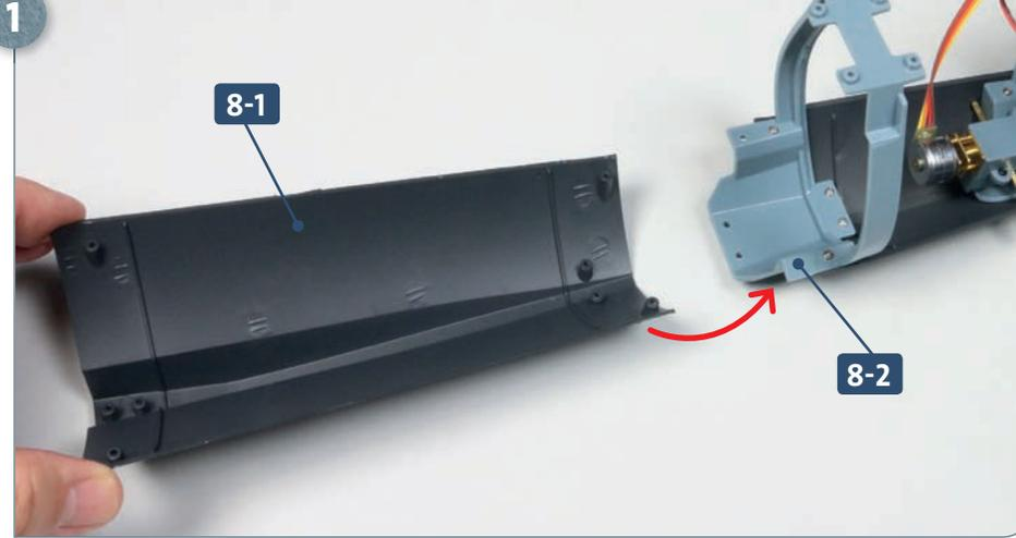
Take the lower hull section **8-1** and fit it onto the connector **8-2**, as shown.
