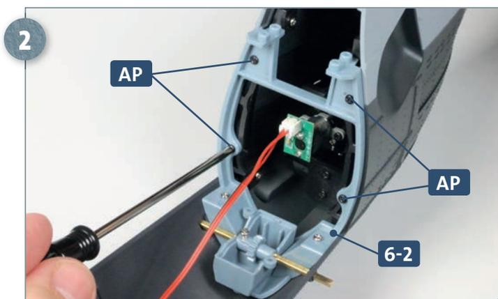
Fix in place using four **AP** screws.
