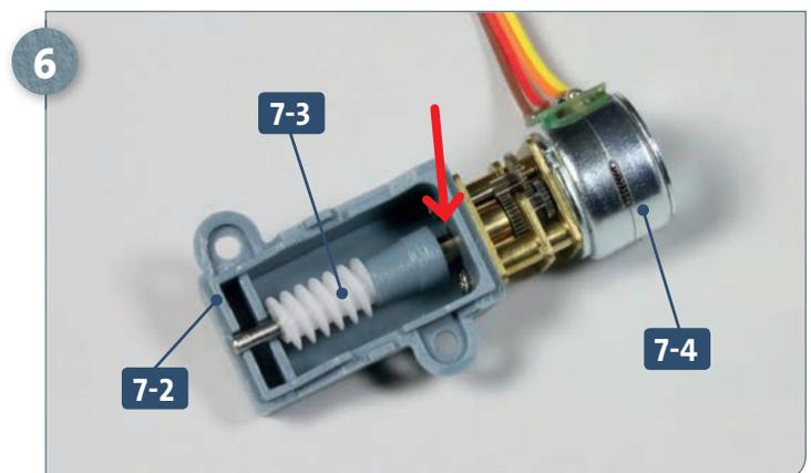
The worm gear **7-3** is correctly seated in the housing **7-2** when its shaft rests within the recess of the case and the other end fits over the shaft of the motor **7-4** (see arrow).
