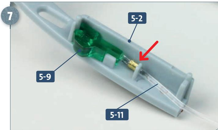
Fit the front end of the first cable 5-11 into the back of the starboard (R) navigation light 5-9, so that the cable clamp (see arrow) sits in front of the tab in the platform 5-2, as shown above.
