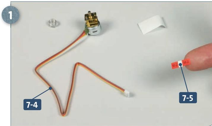
Place the motor **7-4** and cable label **7-5** on your work surface. Remove the wrapper from the motor cable and detach the backing film from the cable label.
