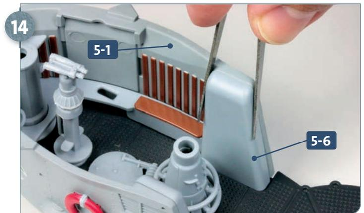
Take the air duct cover 5-6 and apply a little glue to the raised sockets on the back and secure it in place on the starboard (R) bulwark 5-1, as shown.
