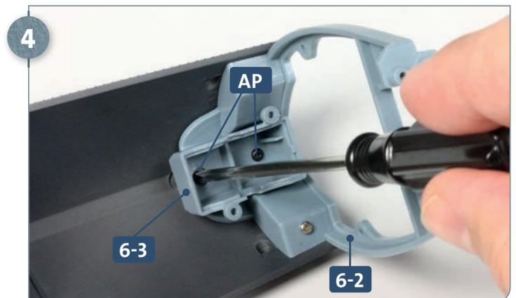
Attach the hydroplane box **6-3** to the connector **6-2** using two **AP** screws.
