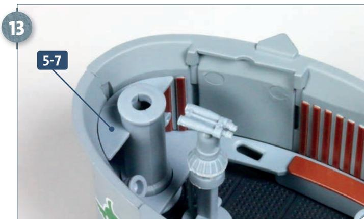
The canopy 5-7 is mounted at the front of the conning tower.
