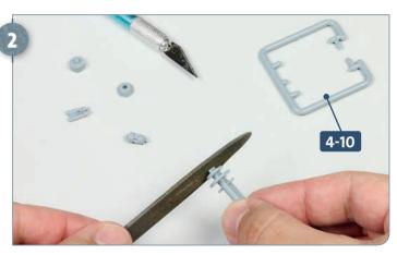
Carefully detach the five pieces from **4-10** and use a small flat file to remove the remains of the frame.
