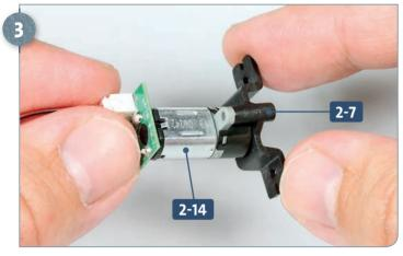
Take the motor support bracket **2-7** and fit its central hole over the hub of the motor **2-14**, as shown.
